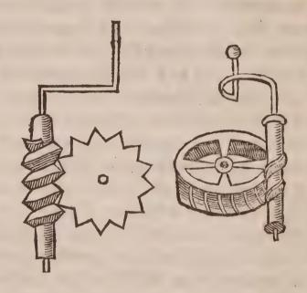
It is used in some Watches. For the composure of which, instead of the female, or concave screw, there must be a little wheel, with some notches in it, equivalent to teeth, by which the other may take hold of it, and turn it round, as in these other figures.
